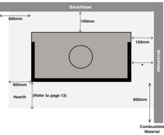
A minimum 110mm solid brick/hebel thick wall should extend a minimum height of 1800mm from the hearth when using a triple skin flue kit or to the ceiling when using a single skin flue kit.
