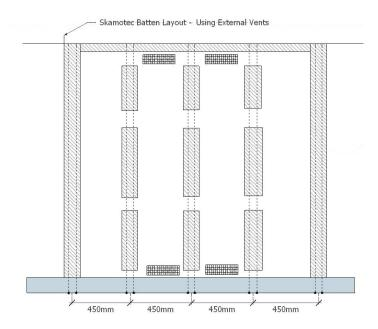
The minimum concealed surface area of vent is one 720cm2 top (9cm  $\times$  80cm) at the top and bottom or 2  $\times$  360cm2 (9cm  $\times$  40cm) top and bottom as illustrated
