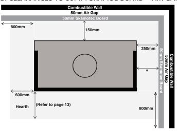
The Skamol boards should extend to a minimum height of 1800mm from the hearth when using a triple skin flue kit OR all the way to the ceiling when using a single skin flue kit (refer to page 17). When using Skamotec board with a 50mm air gap behind, it must also be ventilated for natural air flow circulation, (refer to page 15 & 16 for ventilation requirements).
