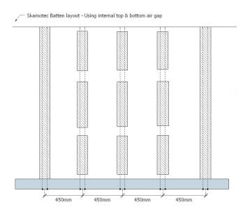
The 25mm top and bottom air gap must extend the full width of the Skamotec cavity and can be left open to create a shadow line effect, or alternatively can be faced with a metal grill/vent
