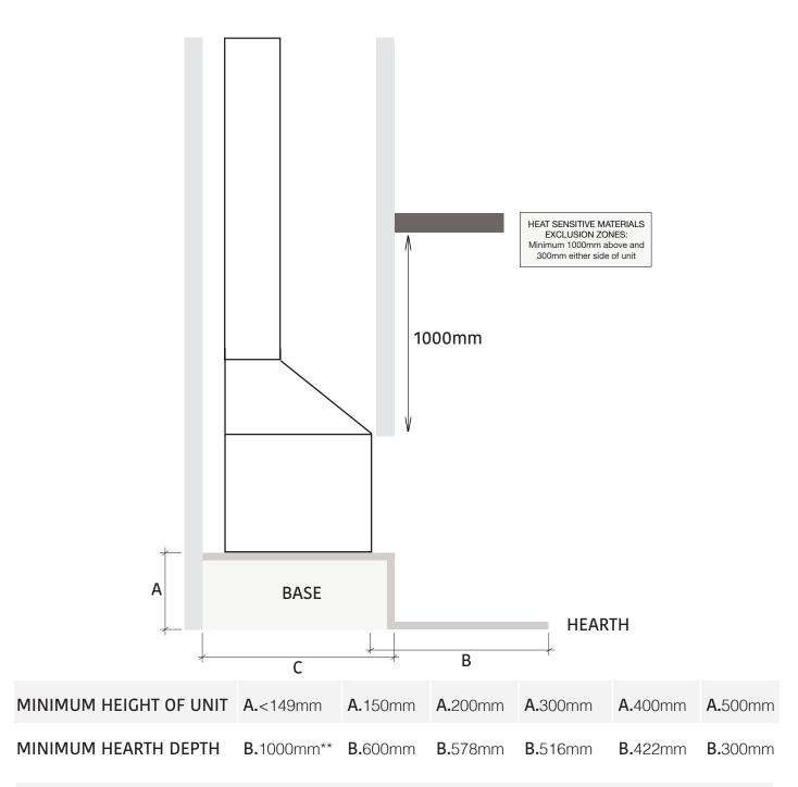
MINIMUM BASE SIZE: WIDTH: 900mm x DEPTH: As per above (C) x THICKNESS: \*150mm MINIMUM HEARTH SIZE: WIDTH: 2146mm x DEPTH: As per above (B) x THICKNESS: \*24mm The unit must be placed centrally in the 2146mm width hearth
