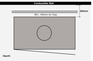
Rear shield must be a minimum 1000mm wide by 900mm high.
