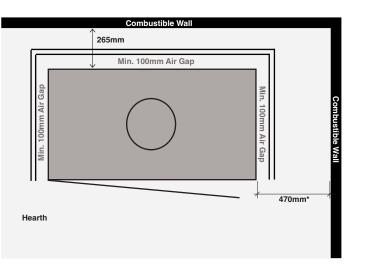
The shield must be a minimum 900mm high, and extend no less than the front of the unit.
