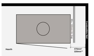
\*The shield must form an abutment with the rear wall and extend no less than the front of the unit, with a minimum height of 900mm.
